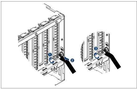
Figure 10: Installing a protective earth conductor
